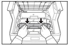
Push down on the top of the toner container to install it firmly in place.
